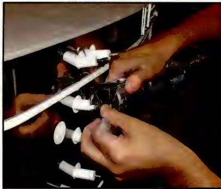
Crimping high temp connector on pigtail
