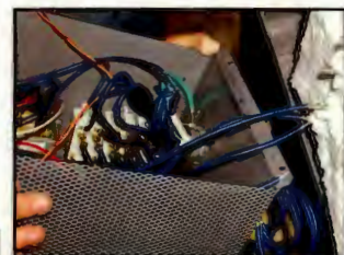
Removing screws attaching electrical box to kiln and gently pulling box away
