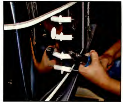
Cutting pigtail to connect to high temp connectors
