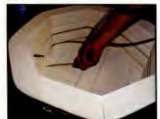
Element pigtail inserted into the hole of the terminal brick
