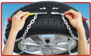
3 Pick up the ends of the flexible cable and join them together on the top of the trye. Try to keep the chain links in front of your hands as in the photo so they do not drop behind the back of the wheel.
