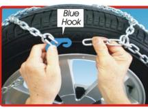
4 Join the side chain & blue hook together on the top sidewall of the trye
