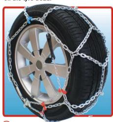
(11) To remove the chains stop each wheel in the same position the chains were fitted, with the autolock lever at the bottom of the wheel as in the photo, then reverse the installation steps in order.
