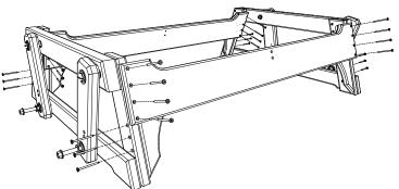
2.Attach (G) Crosspiece Support to Front-Back Crosspieces using 2 - 2" Screws per side, be sure to match all numbers & or letters.
