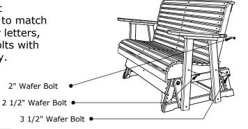
8. Attach (H) Lintels to Armrest Assemblies using 4 - 2" Screws per side, be sure to match all numbers & or letters.
