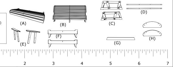
1. Attach (F) Front-Back Crosspieces to (C) Glider Base's Using 14 - 2" Screws per side, be sure to match all numbers & or letters.
