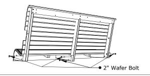
7. Attach Back-Seat Assembly to Armrests using
