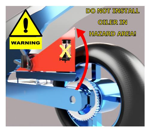
Remember the suspension will compress even further than normal when taking a pillion passenger, the bike is loaded with luggage or when riding over speed humps!
