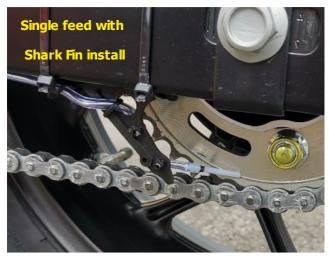
**Note** that the tip of the nozzle is resting on the inside lip or recess that surrounds the teeth of the sprocket.
