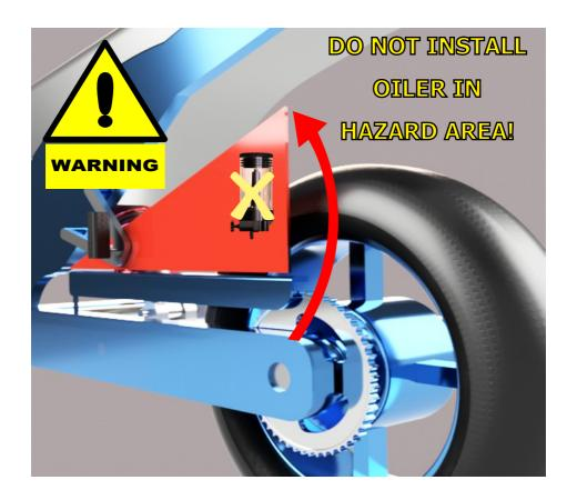
Remember the suspension will compress even further than normal when taking a pillion passenger, the bike is loaded with luggage or when riding over speed humps!
