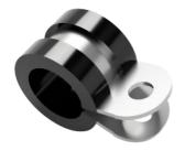
The P Clip is the ideal method to attach the oiler to a round bar frame and provides a rigid secure install. Do not use the multi-fit bracket on small diameter bar frames (less than 30mm diameter) - it will not hold the Auto rigidly enough and may prevent the Auto from functioning properly
