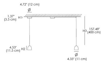
Suspension lamp system crafted in brass. Features a high-luminance LED light source.
