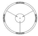
Pendant lamp in aluminum featuring a ring design. The light source employs LED floodlight modules, which deliver uniform illumination. Finish: matte bronze. Dimmer.
