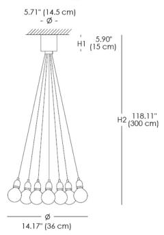
Multiple suspension lamp, available with 7, 13 or 19 points of light. Ilde Wood Max S is made of oak, and features a brown textile cable. This is an UL Certified Lamp.
