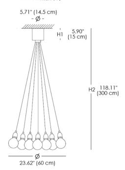
Multiple suspension lamp, available with 7, 13 or 19 points of light. Ilde Wood Max S is made of oak, and features a brown textile cable. This is an UL Certified Lamp.
