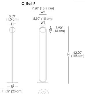
Decorative floor lamp consisting of an opal glass sphere and metal components finished in satin brass or matte black. This is a UL Certified lamp.
