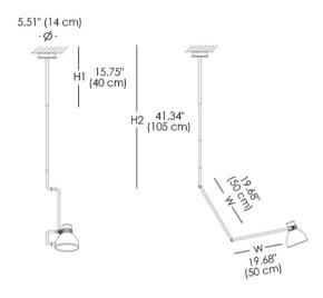
Articulated ceiling lamp designed in the late 70s, in the style of the English school. The simplicity of its forms is reflected in its friction swivel joints and aluminum shade.
