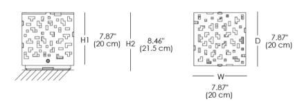
Range of outdoor lamps with geometric forms. Made from corten steel or 316L stainless steel.
