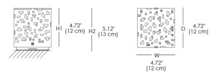
Range of outdoor lamps with geometric forms. Made from corten steel or 316L stainless steel.
