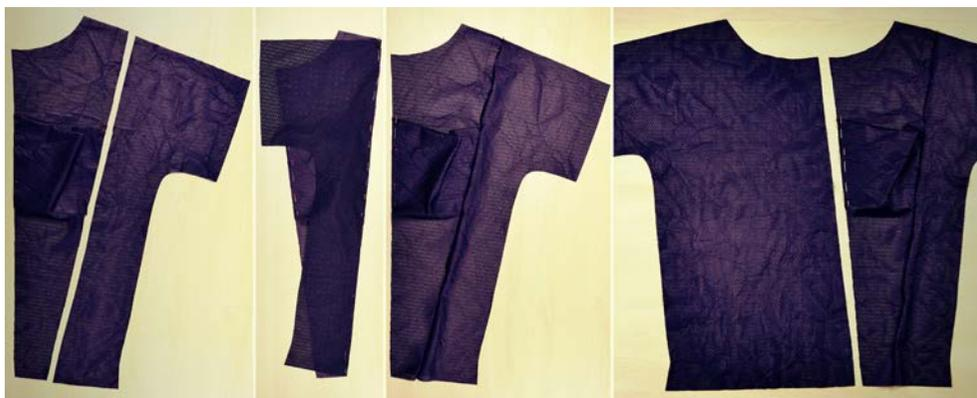
Change threads to a different color and sew three elements in a front together using an overlock machine; now sew up a front with a back on the shoulders and sides, same as in a lining. Note to sew carefully on curves under an arm hole.
