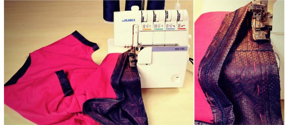
Now it is time for a precise task – you must cut an excess of a material; if you want to avoid it and make a seam so as to cover the edge of a material with a cover-stitch, add smaller allowances on cuffs or cut them before sewing; but then you can't make any mistake; you need to carefully baste the edge of a cuff and sew on a right side, exactly in the place where a material ends underneath.
