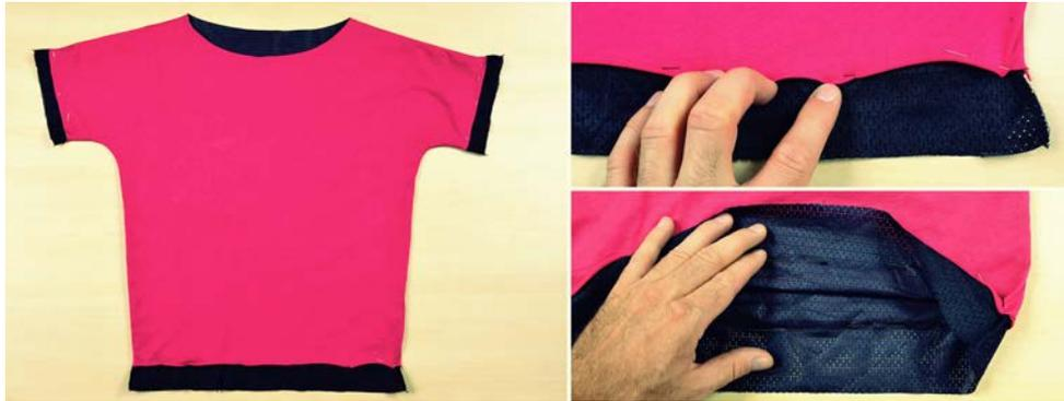
Now fold an allowance of a top material in sleeves and bottom on a lining and pin all 3 layers together (see a picture below); now it is time to trim cuffs using a function of a coverlock stitching; a seam is applied 1.5cm from the edge and should include all 3 layers, closing the edge of a lining inside a cuff; additionally you can baste all edges together, to make sewing with coverlock easier.
