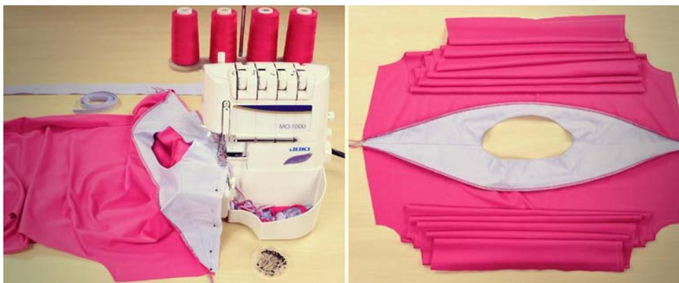
It is time for cuffs. Press them lengthwise in half with an iron and pin on the left side of a dress, so that unhemmed edges of cuffs come in contact with edges of sleeves.
