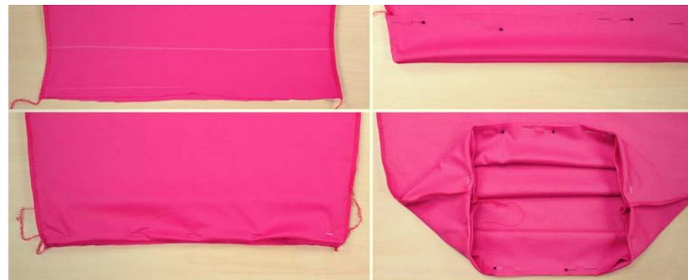
Using an overlock machine, sew a bottom edge (3 layers of a material) by cutting only a small fragment so as not to decrease a binding. Tie the end of an overlock seam and attach manually to the allowance. Turn a binding back down and press the allowance with an iron.
