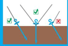
Bluescrew can resist a number of forces from different directions simultaneously. The unique helix is designed to use the weight of the ground for resistance.
