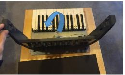
Slide the towel or foam sheet up under the front panel of the synth and lay the panel flat so that it is upside down and pointing towards you:
