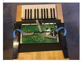
9) With the side panels removed, rotate the control panel to a vertical position to allow access to the keyboard cables.
