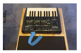
5) Slowly lift the sides and front panel up and away from the keybed. The ribbon cables will remain attached for now.
