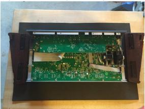
13) Place one side panel onto the synth body as shown. The fit may be very tight depending on the bracket fit. This is normal. If the fit is tight, begin placing the front-most side panel into position, with the rear lifted up at angle. Then apply a constant pressure to the rear to slide it down into place.
