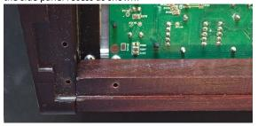
17) Flip the synth over, and check the alignment of the front rail with the front panel. The front rail should fit flush against the panel.
