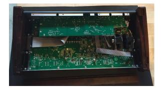
16) With the side panels attached, carefully slide the front wood rail into place. The fit should be tight. Again slightly insert one end, then push the other end into place. The bottom recessed portion of the front rail should align with the side panel recess as shown:
