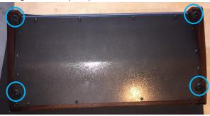
26) Flip your newly transformed SkiniBrute over and test the alignment on a flat surface. Your SB will likely be off balance...and wobble between two of the feet. This is normal and is due to the tolerance of the brackets, side panel mortises, and installation. Four washers are supplied as shims. Carefully inspect how the synth is wobbling..one of the two feet on one side will be lower/higher than the other. Remove the rubber foot and place a washer around the hole as shown:
