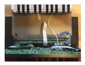
10) Carefully unplug the large keyboard ribbon cable, and small keyboard after-touch cable as indicated below. A small flat screw driver might prove handy to pry the connectors loose.
