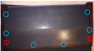
24) Return to the rear screws attaching the bottom cover to the synth and completely tighten. 25) Finally, using the larger wood screws, attach the four rubber feet to the side panels as shown. Be careful not to overtighten and strip the pilot holes.
