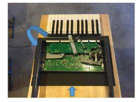
7) Remove and save the 8 self-tapping screws attaching the side panels circled in the photo below:
