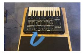
5) Slowly lift the sides and front panel up and away from the keybed. Note the ribbon cables will remain attached.
