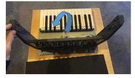
6) Slide the towel or foam sheet up under the front panel of the synth and lay the panel flat so that it is upside down and pointing towards you:
