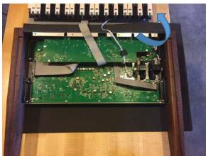
16) Holding the keybed to the front panel, carefully flip the synth back upside down and lay on the towel or foam sheet.
