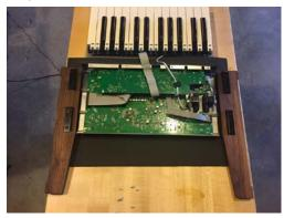
10) Working on one side at a time, position the side panel sliding the brackets to the back of the synth as far as possible, and tightly into the synth body. Try to maintain pressure on the panel in these directions while inserting the screws. It's ok if the bracket holes may look misaligned at this point. Insert one of the middle self-tapping screws just enough to engage the threads. Do not tighten.
