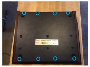
19) Using the black wood screws included with your new side panels, insert and tighten the 8 screws circled below. Do not over tighten. Note the pilot holes in the side panels may not align perfectly to the bottom panel holes. Do not worry, the screws will eventually seat into the pilot holes as they are tightened.
