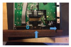
11) Continuing to apply pressure towards the side and back of the synth, thread the remaining self-tapping screws.
