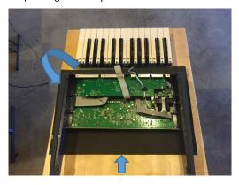
7) Remove and save the 8 self-tapping screws attaching the side panels circled in the photo below:
