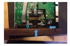
11) Continuing to apply pressure towards the side and back of the synth, thread the remaining self-tapping screws.
