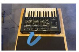
Slowly lift the sides and front panel up and away from the keybed. Note the ribbon cables will remain attached.
