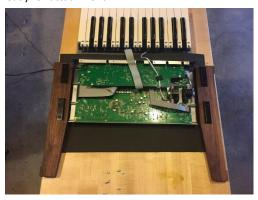
10) Working on one side at a time, position the side panel sliding the brackets to the front of the synth as far as possible, and tightly into the synth body. Try to maintain pressure on the panel in these directions while inserting the screws. It's ok if the bracket holes may look misaligned at this point. Insert one of the middle self-tapping screws just enough to engage the threads. Do not tighten.
