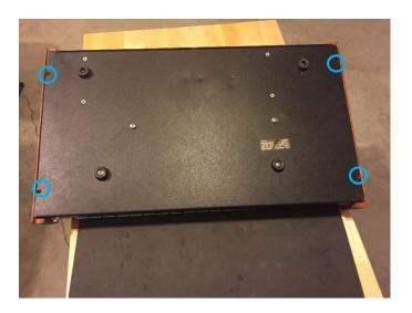
19) Allow the adhesive to cure for the time specified by the adhesive manufacturer. For silicone adhesive this is usually 24-48 hours. If desired, once cured, you can open the synth back up and clip the excess length of the installed spacers.
