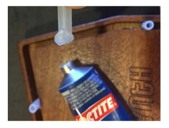
3) Arrange the spacers as in the photo below; two on the top section, and one in each section on the back. Allow the adhesive a couple of hours to set.
