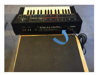
8) Rotate the front panel straight up from the keys, then towards the back, resting it pointing straight up.
