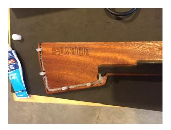
16) Repeating the procedure from the test fit, firmly press the side panels onto the synth top panel.
