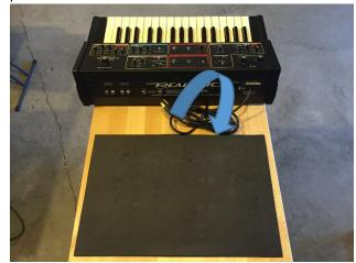
Flip the synth over towards you and remove the four bottom side panel screws.
