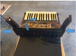
17) With the side panels in place, rotate the synth assembly back onto the keybed. You'll have to lift the rear panel up to slide then synth onto the keybed.
