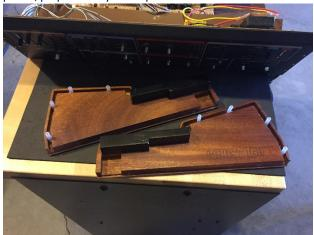
11) Slide each panel on the synth, fitting them so that the spacers are to the inside of the panel. The top panel should just slide between the spacer and outer wall of the channel.
