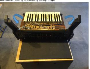
9) Pry each side panel loose from the top panels. The panels are secured with a flexible epoxy. This can take some back-and-forth wiggling but it shouldn't require excessive force.
