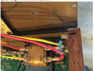
13) Once in place, the panels should have a snug fit due to the spacers. Rotate the entire synth assembly back onto the keyboard. You'll have to lift the rear panel up to slide the synth onto the keybed.
