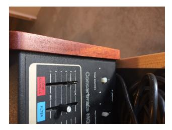
14) With both panels dry fitted, flip the synth back over and adjust the alignment to the bottom panel. This might require pulling the panels back out slightly from the front panel. The bottom panel should fit snuggly against the side panel lower edges.
