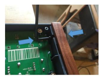
16) Proceeding to the work toward the rear, thread the next screw and fully tighten. You can use the Allen wrench length-wise and run the tool over or under the ribbon cable.
