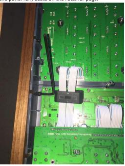
20) Finally, thread and fully tighten the rear screw.
