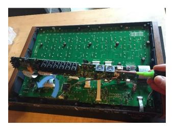
7) Using a Phillips head screw driver carefully remove the two (2) rear screws from each side panel, as shown below. Take special care not to scratch the circuit board. The screws are firmly seated into the plasti-wood panel. You'll have to supply lots of pressure to the side of the instrument in order to get the screws starting to rotate.
