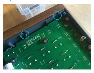
10) You're going to only partially loosen each screw a little at a time. As you do this, the side panel will become loose and can be pulled slightly away from the instrument as shown below:
