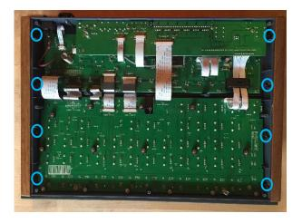
5) In order to remove the screws towards the rear, first remove and save the five (5) screws securing the upper jack plate circuit board as shown below:
