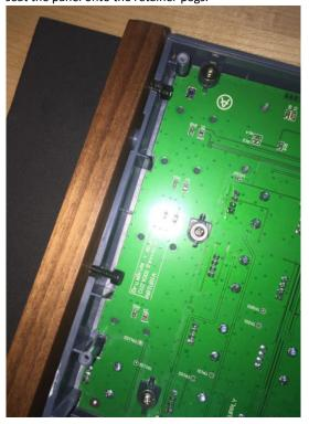
19) Fully tighten these front two screws. Proceeding to the third screw to the rear, thread and fully tighten. Make sure the panel fully seats on the retainer pegs.
