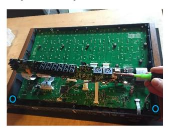
On the screw at the right side of the instrument (near the power switch) it may be easier to work with the screwdriver under the power wires as shown:
