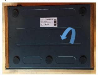
4) With DB opened, we can get a good look at our goal: to remove the eight (8) screws securing the instrument's plasti-wood sides. The two screws towards the front of the instrument are the hardest to access, so we'll approach those last once we've achieved some wiggle room. If you work carefully, you can avoid having to unplug any connectors.
