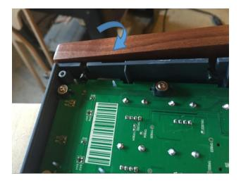
15) Now, completely tighten the front two screws using a 3mm Allen Wrench. As you tighten, make sure the panel is fully seating onto the retainer pegs. Also, be careful not to damage the circuit board with the tool. The screws have been located higher on the GMUSynth panels to allow easier access than the originals.
