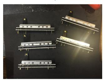
21) The adapters include holes for daisy chaining power for the LEDS. Each side of the adapter includes a positive and ground that is repeated on the opposite side. These are intented to be wired together with a jumper soldered into the top of the PCB (which are plated holes.) Right angle connectors can be used for wiring in SIL connectors for connecting between boards.
