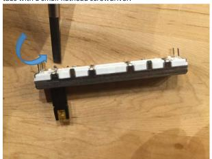
12) Once bent away from the body, use needle nose pliers to complete a 180° bend so the tab is now pointing away from the slider.
