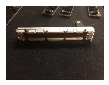
13) Next, fit the modified PTL slider into the top of the adapter board. They only fit in one direction. Using a block of wood or edge of a bench, lay the sliders upside down with the shaft pushed all the way to one side.
