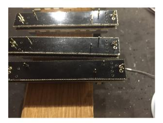
18) Inspect the assembly for board alignment. If necessary, re-wet the pin and adjust the fit.
