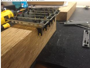
14) Solder in the PTL pins to the adapter board.
