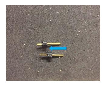
5) Now, using the Spacer as a jig, insert the double pins into each set of double holes on the ends of the spacer board. Insert the
