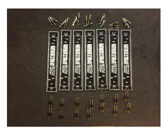
3) Note if you need to cut pins from a row of SIL header pins, the easiest way is as follows: Hold the group of pins you are cutting, squeezing the long side of the pins firmly between your fingers. Using the cross cutters, snip about half way through the v-scored notch on the pin row. This will leave the pin body intact, and prevent the cut pin from shooting out of sight.
