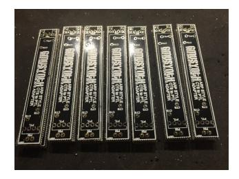
Once the adapters are fitted on top of the pins, proceed with soldering in all seven pins into the adapter boards.
