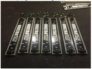
6) Insert the single pins into the holes labeled CTS, inserting the LONG side of the pin into the foam. Try to insure the pins are vertically straight and not leaning.
