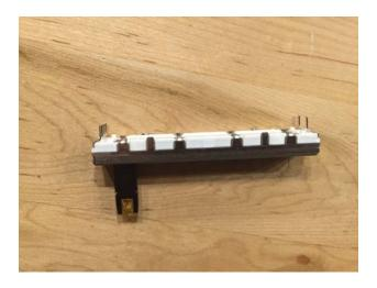
11) With the PTL slider laying on its side with the four pins to your left and shaft pointing towards you, pry open the lower retainer tabs with a small flathead screwdriver.
