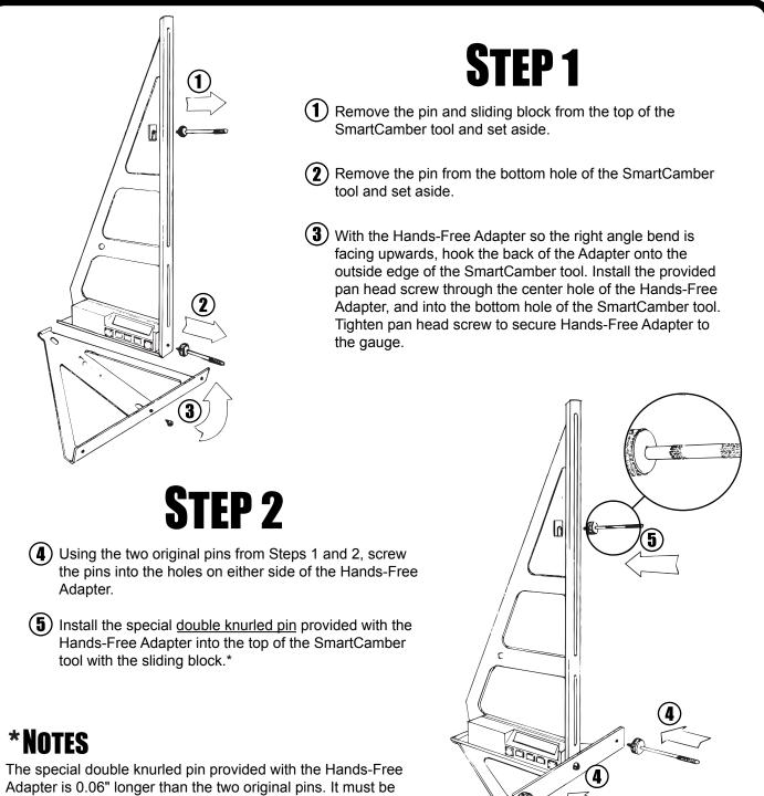
Adapter is 0.06" longer than the two original pins. It must be installed at the top of the SmartCamber tool to keep the tool properly calibrated (it offsets the thickness of the Hands-Free Adapter). Use a piece of tape on the wheel so the Hands-Free Adapter pins will not score the wheel.
