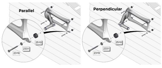
Step B12 Tighten the four  $1/4 \times 2$ -1/2 inch Hex Head Lag Screws (2319) with a 7/16 inch wrench. **Do not over tighten.**
