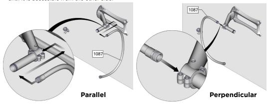
**Step 14** - Install the Flange Assembly onto the axle with the crank handle to the outside.
