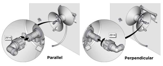
**Step 17 -** Attach the Swivel to the axle. Hand tighten firmly.
