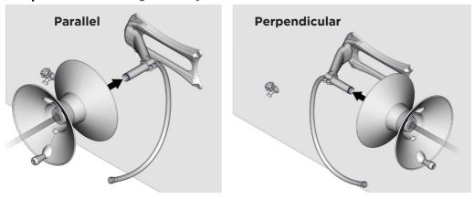
**Step 15** - Install the Cam-lever Brake (2587) onto the axle. **Note:** Align the tab on the brake with the notch in the flange.
