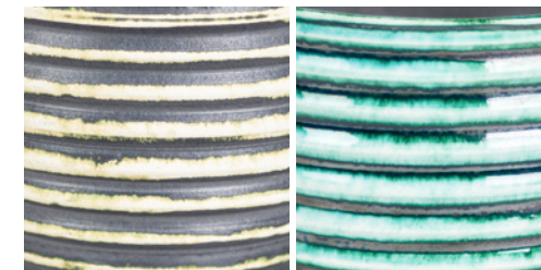
One coat wiped back One coat wiped back under clear glaze (S-2101 Crystal Clear Brushing)
