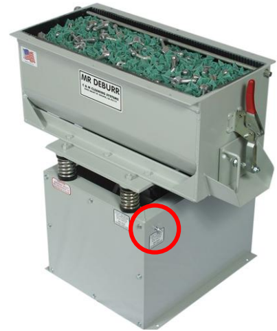
Figure 3: Bearing Grease Zerk Fitting Circled
