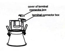
Open the cover of terminal connector box as drawing2.
