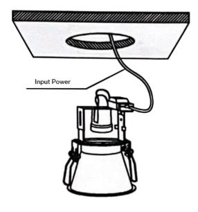
Connect the input electrical wires to the terminal connector, fix the erminal connector box's cover as drawing 3.
