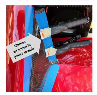
**Step 2:** Clean off remaining tape residue from the vertical bond line area by using a blade or other sturdy object to scrap away the residue. This area should be as clear of tape as possible. Remove any bulk tape residue from the triangular rear tape patch. It is not critical to fully remove tape from the triangular pad, as new tape will not bond over it.
