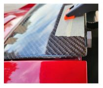
Left: Detail of the carbon panel sitting on the shims while aligning. The front edge of the panel and the car body should be co-linear.
