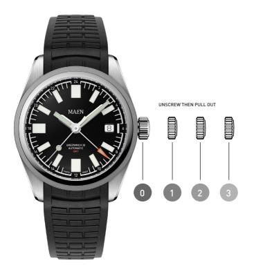
To screw the crown back down against the case, return it to position 1 and apply light pressure on it while screwing it down clockwise against the case.
