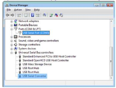
Perform a loopback test by using CommFront's 232Analyzer software: Connect a USB-TTL converter to your USB port, short pin TX (TTL Out) to RX (TTL In) on the termination board, and then send commands from the 232Analyzer software. You should receive an echo of the commands sent. By performing a simple loopback test like this, you can test both the transmitter and receiver of the USB-TTL converter. This is very helpful when you are in doubt about the performance of your converter.
