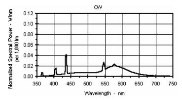
**FIGURE 1** Spectral power distribution curve supplied by the fabricant for the F34CW/SS/ECO/CVP white fluorescent lamps in the work place. They were composed of T12 bulb of 34W with a color temperature of 4100 K.
