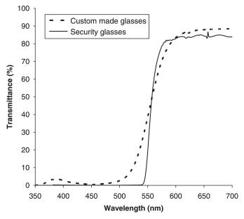
**FIGURE 2** Transmittance level of the two optical filters used. The blue-blocking security glasses (——) allow passage of 0.1% of light of wavelengths  $<540\,$  nm, 40% at  $555\,$  nm, and 82%  $>600\,$  nm. The custom-made, blue-blockers (- - - -) allow 3.5% of the  $387\,$  nm light to pass through, then allow passage of 0.5% of the light at  $450\,$  nm, 25% at  $540\,$  nm, 45% at  $555\,$  nm, and 83%  $>600\,$  nm.
