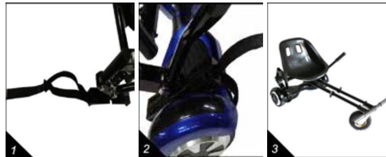
Step 5. Fasten the Strips to the Balance board
