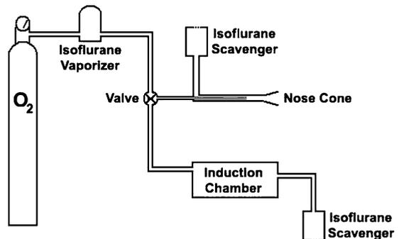
**Fig. 2** Schematic of the Isoflurane Anesthesia Setup. A schematic diagram of the flow pattern of anesthetic gas for the mouse ERG. A 2% mixture of isoflurane vapor in oxygen flowing at a rate of 0.9 LPM can be directed either to an induction chamber, or to a nose cone on the ERG warming platform (see Fig. 1). Both the induction chamber and the nose cone are exhausted through scavenging canisters to remove isoflurane vapors before venting the air back into the general circulation
