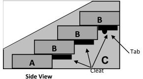
Repeat the same process to glue side wall **D** to the step assembly. Once assembled the steps should look like the photo at the beginning of this section.
