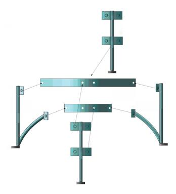
With Fire Pro 900 Stand => all completed when screwing 16 bolts and 16 nuts. Insert bowl into top ring.
