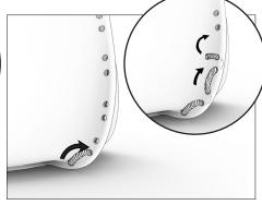
3. Thread the rope through the next hole above and pull towards the internal of the pot. Thread the rope in alternating in-out pattern as illustrated. CAUTION: Do not over tighten, but ensure
