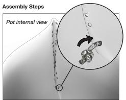
1. Locate the last hole on one side of the pot. Tie a simple knot on the end of one of the ropes and thread unknotted end through hole.
