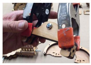
24. Apply glue to the mating surfaces of the Left Side Fender Assembly and install onto Frame 25. Install Right Side Fender Assembly and lightly clamp Fenders to Frame. Set aside to dry.
