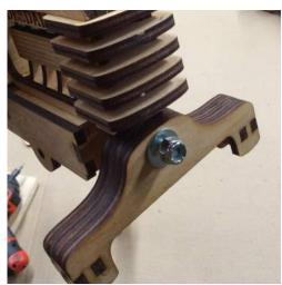
32. Slide the Frame Rear Cover Plate onto the threaded rod and secure with a flat washer and nylon lock nut. Use pliers to grasp the threaded rod through the access hole in the Frame while tightening the lock nut with a 7/16" wrench or deep socket. (Caution! Do not over-tighten the lock nut—you can crush the frame!)
