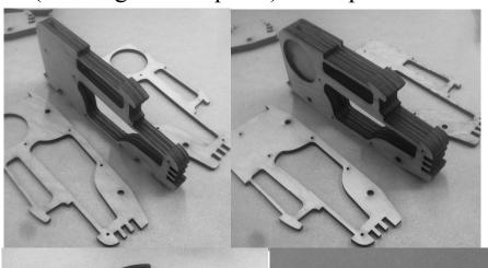
5. Stack the remaining four body profiles (two on each side of the center stack) as shown. Do not use glue.
