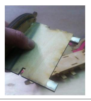
Assemble Rumble Seat Back components as shown. Ensure that the parts are arranged in the proper order on the Left Hand side and the Right Hand side. Seat Back Profile with the tab goes in the middle, and the smaller Seat Back Profile goes on the inside to create the ledge for the flexible Seat Back Outer Panel. Do a "dry" test-fit to ensure proper spacing and alignment.
