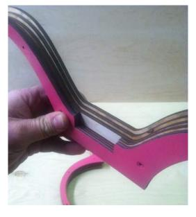
Arrange fender parts in LH and RH stacks.
