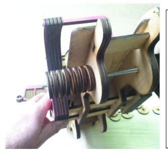
Insert Spokes on both sides of each Wheel. Slide onto axle with 7 Hub Spacers next to the Frame and 1 Flat washer on the outside of the Wheel. Install opposite Wheel and Spokes, Hub Spacers and Flat washer. Then secure with Axle Nuts.
