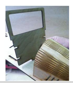
Glue and Assemble Engine Compartment Cover to Floorpan. Set Windshield Firewall component in place (no glue). Set Back Wall in place (no glue). Apply glue to edges of Windshield, Floorpan, and Back Wall as shown.
