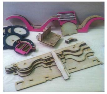
Assemble Frame components: 4Frame Rails, 2-long Frame Crossmembers, 2-short Frame Crossmembers, and Floorpan.
