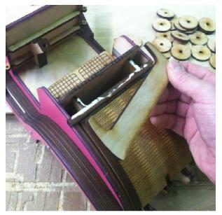
Re-install #6 screws in pivot holes for Rumble Seat Back. The Rumble Seat Back should now lift the Rumble Seat Bottom when it is opened. Sand corners and mating surfaces if it does not operate smoothly.
