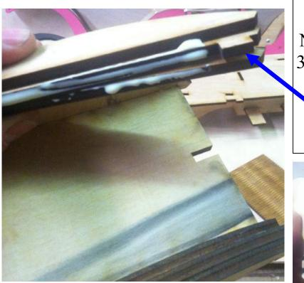
Now glue and assemble the 3 Center Seat Back Profiles. The profile with the extra tab goes in the middle.
