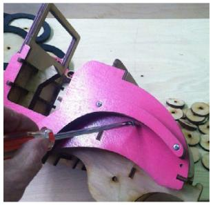
Partially install one #6 screw in hole under rear fender as shown. Insert Rumble Seat Bottom and install #6 screw in opposite side hole. The Rumble Seat Bottom should pivot freely. Slightly enlarge pivot holes in Side Panels if necessary.
