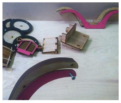
Now remove screws from Fender Sub-Assemblies. Align LH and RH Outer Fender Profiles on each Fender sub-assembly and reinstall screws. Glue is not necessary.
