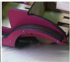
Assemble LH and RH Fenders on each side of the vehicle. Glue is not necessary, but can be applied to the slotted areas if desired.
