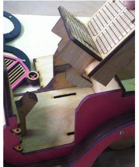
Install the Seat sub-Assembly by inserting the hooks into the Floorpan and sliding the assembly back into place. (no glue)
