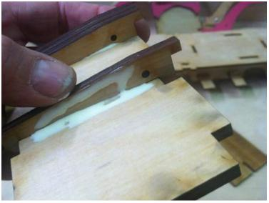
Assemble and glue Rumble Seat Bottom components as shown. (9 ribs, 1 Seat Bottom panel, 1 Seat Front Edge)
