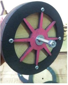
Remove screws from Wheel-halves. Place two halves back-to-back and install four screws, as shown.
