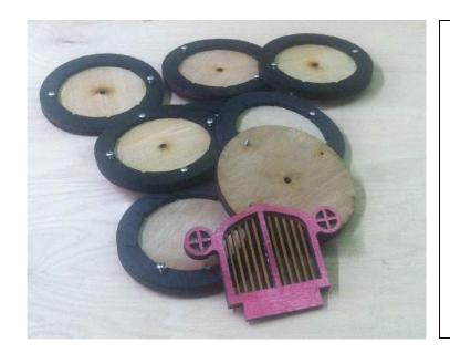
Glue Wheel Tread Rim (8) to Solid Wheel (8). Align screw holes and install two screws to clamp parts together. These 8 Wheel-Halves will be assembled into 4 Wheels in Section Two. Set aside to dry.
