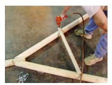
7. From machine bolt, measure 32" down swing leg. At this location, use 4" lag bolts to secure two of the 35" braces to swing legs. Use a 1/4" washer when inserting each 4" lag bolt.
