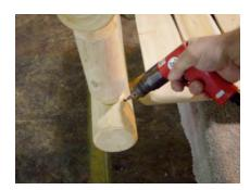
5. Install 2" screw where all doweled ends were inserted, securing seat and seat back to arm assemblies.
