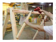
8. Stand frame upright and tighten 7 ½" machine bolts *only enough* to allow frame to stand freely. Measure 24" down from top of the swing leg, and 24" out from end of top pole. At these points, use 4" lag bolts to secure the remaining four braces to the swing (as shown in these two photos). Use ½" washer when inserting each lag bolt. Now, tighten 7½ machine bolts firmly.
