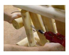
3. Through pre-drilled holes in seat back, use 3 3/8" lag bolts to secure the arms to the seat back (as shown). Use a 5/16 washer when inserting each 3 3/8" lag bolt.
