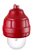
The Federal Signal Model 24XSTHI Explosion Proof Strobe Light produces 80 high-intensity flashes per minute. The 24XSTHI is UL listed for Class 1, Division 1 & 2, Groups C & D; Class 1, Division 2, Groups A, B; Class II, Division 1, Groups E, F & G; and Class III. The 24XSTHI is Type 4X and IP66 rated.
