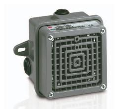
The Model 350WB (AC current) Vibratone® horn produces sound by the electro-mechanical vibration of a stainless steel diaphragm. The horn mechanism with diaphragm is attached to the grille. Indoor or outdoor use is made possible by the water- and dust-tight backbox.
