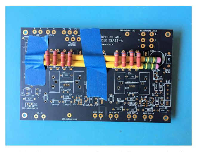
Noir includes eight 3-Watt resistors: R25-28 and R75-78. All eight resistors are 68 ohms. These are the first components to install on the Printed Circuit board.
