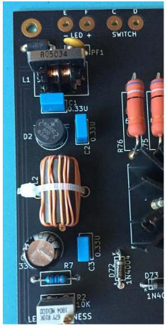
Part 2. Stuff and solder the current regulator diodes D25 and D75. These have an unusual PCB "footprint" with lots of test points and not-used holes nearby. The blue band end ("cathode") of this diode goes into hole 5, and the other end of this diode ("anode") goes into hole 1. Just as shown on the white silkscreened printing on the PCB
