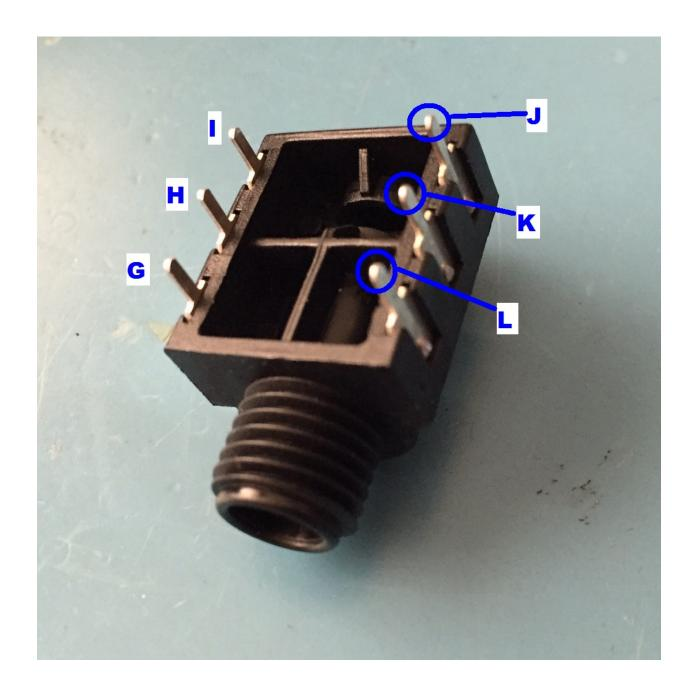
The letters G H I J K L also appear on the printed circuit board, and on the circuit schematic diagram. Check the schematic now, and find them. They tell you how to connect fly-wires between the headphone jack and the Noir printed circuit board. Please print this page of the Build instructions on paper, and keep it nearby on your work bench, as you begin to fly-wire the headphone jack.
