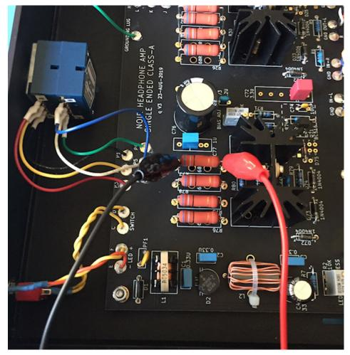
Before the first power-up, twist the knobs of bias trimpots R23 and R73, at least 10 full rotations counter-clockwise ("to the left"). This reduces the bias current so components don't overheat while you're doing the adjustment.
