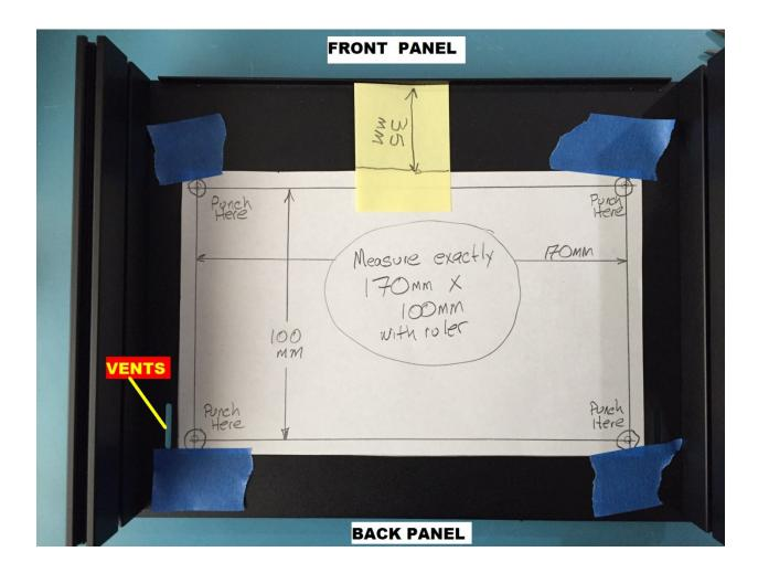
Tape the template to the bottom plate (floor) of the chassis as shown. It should be centered left-to-right, and it should be 35mm from the front panel bent "lip" of the chassis bottom plate.
