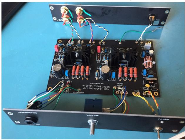
There is one more fly-wire which solders to the PCB and is routed to the rear panel. It has a connection hole on the PCB labeled "GROUNDING LUG". The other end of the fly-wire can either (a) solder directly to the "SHIELD" solder-pad on the inside face of the rear panel (photo on p.29) or (b) solder to a grounding lug as shown below. This lug fits over one of the M4 bolts that attaches the rear panel to the rest of the chassis.
