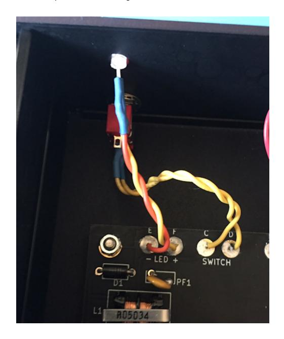
Cut four pieces of wire that are far too long (6 inches). Solder two wires to the terminals of the power switch, and two wires to the terminals of the LED. You can add heatshrink tubing over these joints if you wish.
