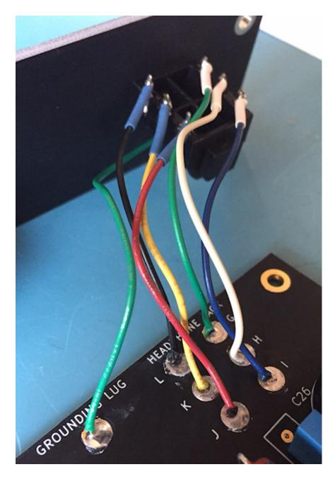
Cut six pieces of wire that are far too long (6 inches). Here I have used six different wire colors, to make it easy to tell them apart in the photos. I soldered a green wire to Neutrik terminal "G", a white wire to "H", a blue wire to "I", a red wire to "J", a yellow wire to "K", and a black wire to "L". You can add heatshrink tubing over these joints if you wish.
