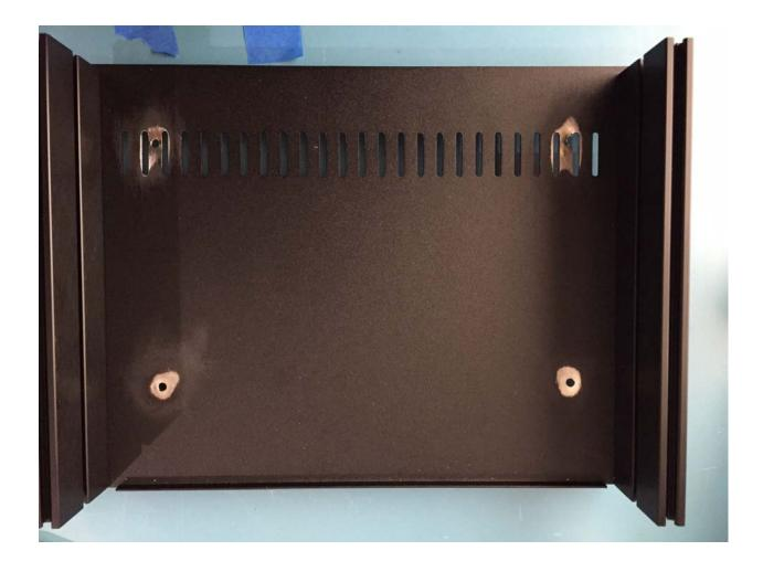
After drilling, use relatively coarse sandpaper to remove the black paint and expose the shiny steel, surrounding the drill holes, on the inside of the chassis. (No need to do it on the outside of the chassis). This exposed metal lets the mounting posts make good electrical contact to the bottom plate, extending the Faraday Cage which surrounds Noir and blocks hum.
