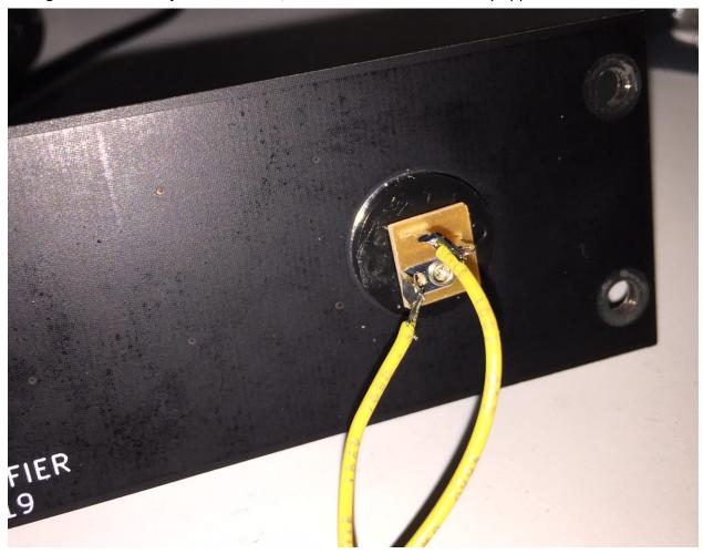
Noir's inputs and preamp-outputs use RCA jacks on the rear panel. The gold plated jacks in the BOM consist of six pieces. They mount to the rear panel as illustrated in these four photos
