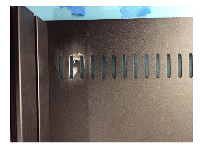
Here's a close-up after drilling and sanding. Please notice that the metal has been deflected (warped!) downward, unfortunately. I put a huge stack of newspapers between the metal and the piece of wood underneath, when drilling. This was a mistake, the newspapers had a lot of "give" but what I wanted was Support. The metal deflected. Oops!
