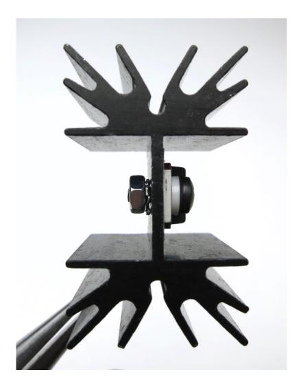
Part 9. Stuff one of the just-completed MOSFET-heatsink assemblies, into position Q72. The silver colored pegs on the bottom of the heatsink, fit into the holes on the PCB labeled "SUPPORT". Using lots of flux and lots of time, solder the two support pegs to the PCB. Then solder the three leads of the MOSFET to the PCB. Trim the MOSFET leads but leave the large support pegs alone.
