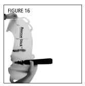
Step 2 - Fold the left cell lobe **under** the right cell lobe at the FOLD#1 line (Fig. 16). Ensure the "Jerk to Inflate" tab is placed beside the cell.
