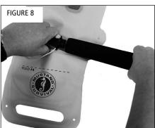
Step 2 - Remove the handle, containing the discharged CO<sub>2</sub> cylinder, by firmly rotating counterclockwise (Fig. 8). To ensure that you do not re-install a used cylinder, discard immediately. If cylinder is discharged, replace with new handle. Ensure the cylinder has not been pierced. See RE-ARMING.
