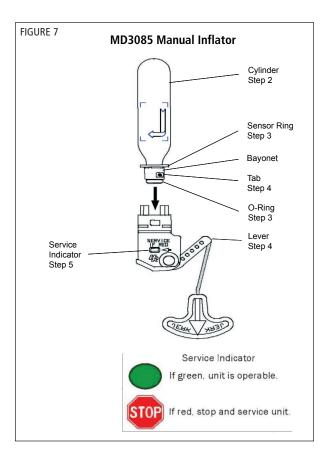
Raise, and hold, the lever into the inflator housing. Install a new cylinder/bayonet assembly by engaging bayonet tabs in housing, pushing in then turning clockwise 1/8 turn to a full stop (Fig. 8).
