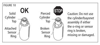
IMPORTANT: You will damage the sensor ring if bobbin and cap are not installed first.
