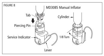
5) Examine the service indicator (Fig. 8) and ensure it is GREEN. If the service indicator is red, the mechanism has been fired or is incorrectly fitted and the inflator requires service. See Re-arming Your PFD (MD3085) p. 8.
