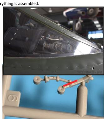
Remove lower light beacon from Port wheel fairing. New part mounts outboard of centreline on starboard fairing.
