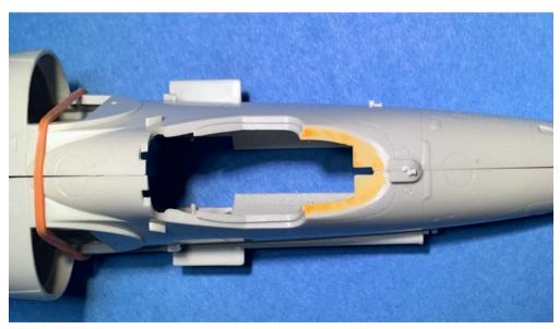
Use a razor saw, hobby knife, or your preferred method, to remove part of the upper fuselage edge (Orange Area in photo) to allow the new IP (Instrument panel) & HUD to fit inside.
