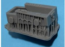
3D printed resin parts are super detailed and accurate however the resin can be brittle and snapping the parts from their printing supports will nearly always leave a 'divot' in the part. This divot may or may-not require filling depending on its
