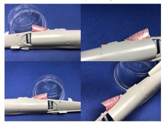
3. Remove upper fuselage anti-collission light mount and flatten out the rounded upper fuselage profile in the red shaded areas.
