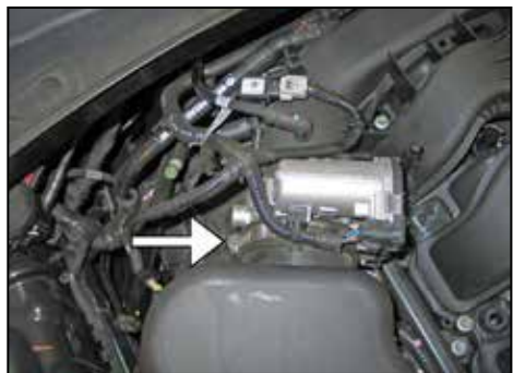
5. Loosen the hose clamp that secures the intake tube to the throttle body.
