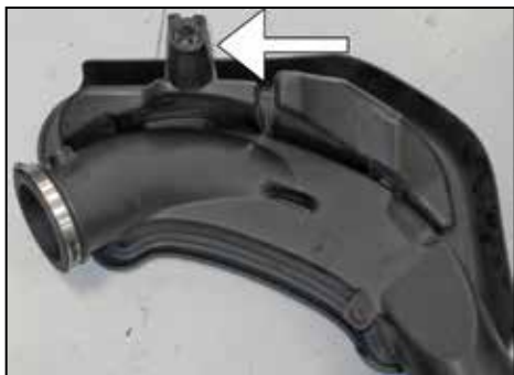
20. Remove the intake plenum mount grommet from the intake plenum.
