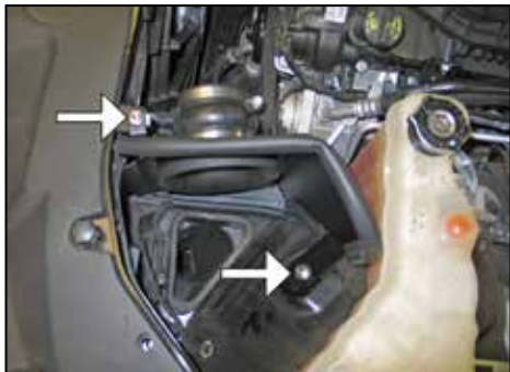
14. Install the heat shield assembly onto the inner fender; secure the mounting bracket to the factory airbox mounting location with the provided hardware. The inserted nut is to be placed in the hole of the inner fender and then secured by tightening the assembly's bolt.
