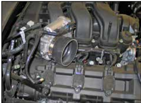
15. Install the provided silicone hose (08690) onto the throttle body and secure with the provided hose clamp.
