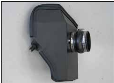
13. Install the silicone hump hose (084057) onto the filter adapter and secure with the provided hose clamp.
