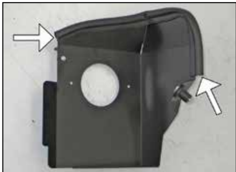
10. Install the provided longer edge trim onto the top of the heat shield as shown. NOTE: trimming of the edge trim will be necessary.
