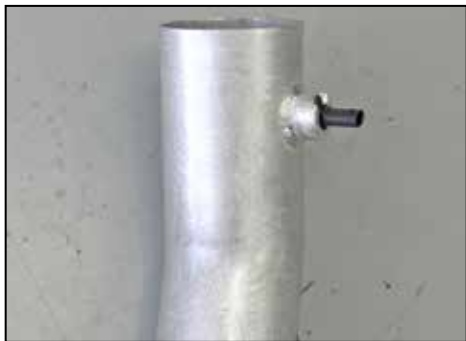
17. Install the inlet air temperature sensor into the K&N® intake tube as shown, turning the sensor clockwise to lock. NOTE: The inlet air temperature sensor is very fragile.
