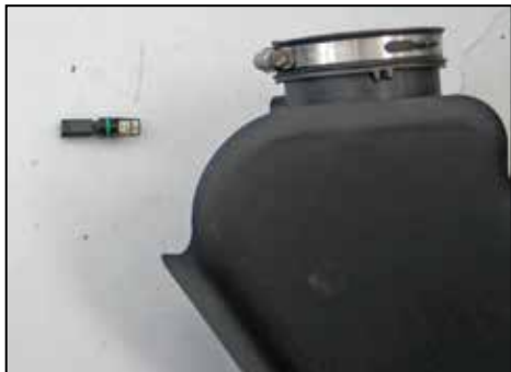
16. Rotate the inlet air temperature sensor counter clockwise and then remove from the factory intake tube. NOTE: The inlet air temperature sensor is very fragile.
