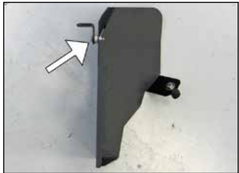
9. Install the heat shield mounting bracket (070066A) onto the heat shield as shown using the provided hardware and spacer.
