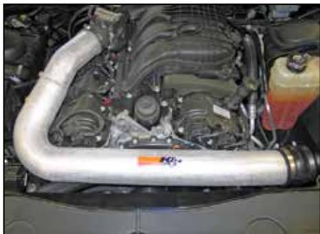
19. Install the K&N® intake tube into the silicone hump hose and then into the silicone hose on the throttle body. NOTE: Do not tighten the hose clamps at this time.
