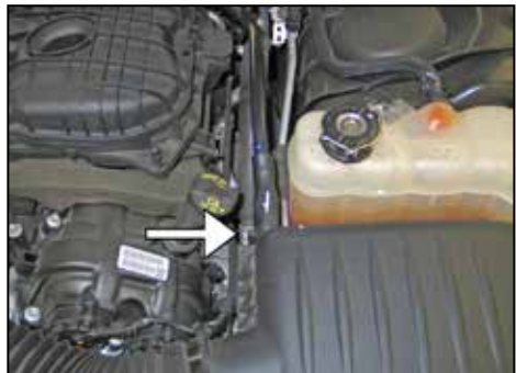
4. Disconnect the crankcase vent hose from the air filter housing. NOTE: On later models the crank case vent line connection will be near the throttle body.
