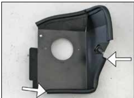
11. Install the provided shorter edge trim onto the bottom of the heat shield as shown. NOTE: trimming of the edge trim will be necessary.
