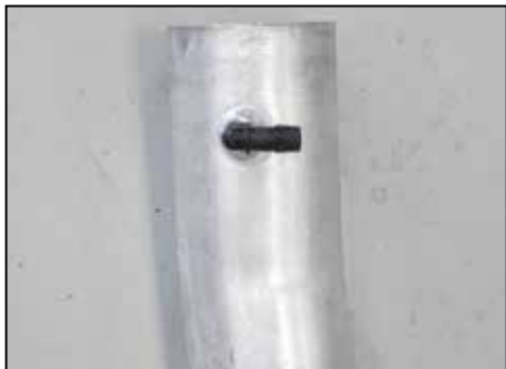
18. Install the 90° NPT fitting into the K&N® intake tube as shown. NOTE: NPT fittings are easy to cross thread. Install the vent fitting “hand” tight, then turn it two complete turns with a wrench.
