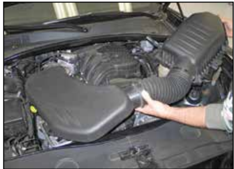
7. Remove the complete stock intake system from the vehicle. NOTE: K&N Engineering, Inc., recommends that customers do not discard factory air intake.
