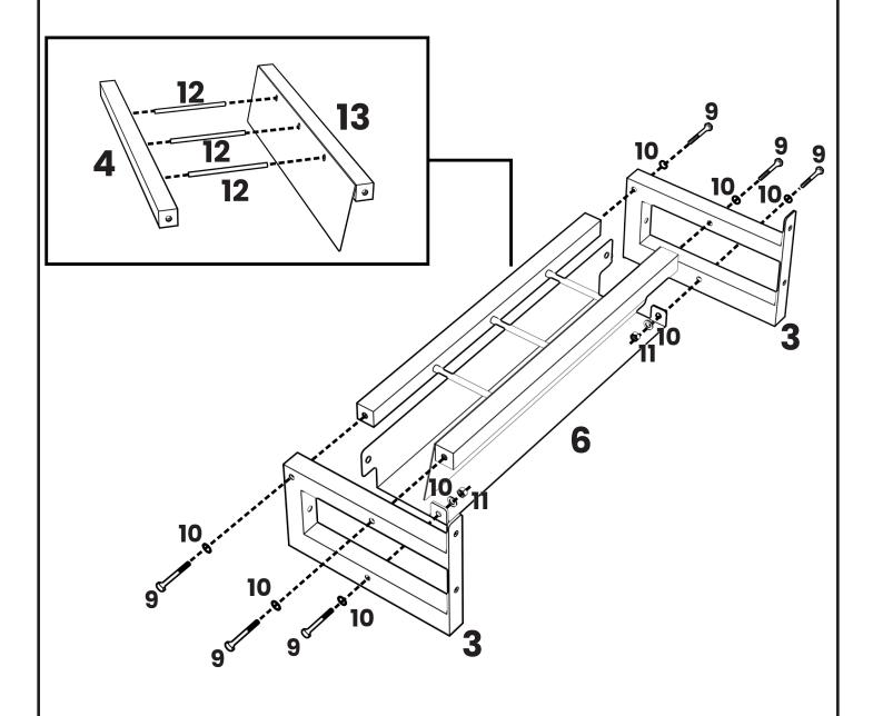
Assemble the bottom bar holder with the divider poles sitting the front and back bottom dividers. Align the two side frames with the floor piece and the bottom bar divider in between. Once aligned tightened as shown above.
