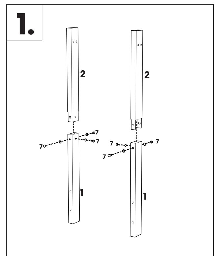
Insert the top uprights into the bottom uprights and secure with the M8X15 Bolts and washers.
